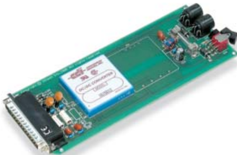
The DBK32A provides additional power for LogBook and Daq systems when the power expansion needs exceed the built-in capacity of the mainframe
